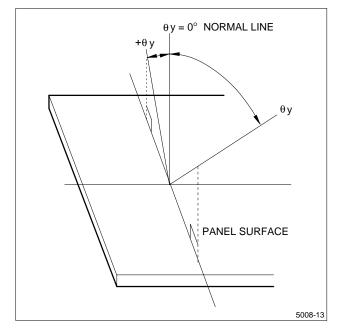
Figure 12. Dot Matrix LCD Viewing Angle
