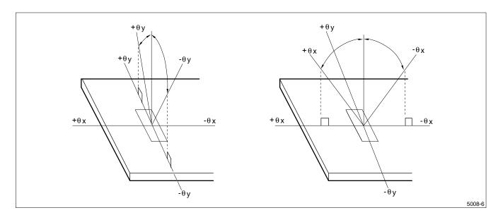
Figure 6. Definition of Viewing Angle
