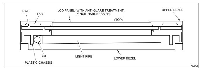
Figure 1. LM64C142 Construction
