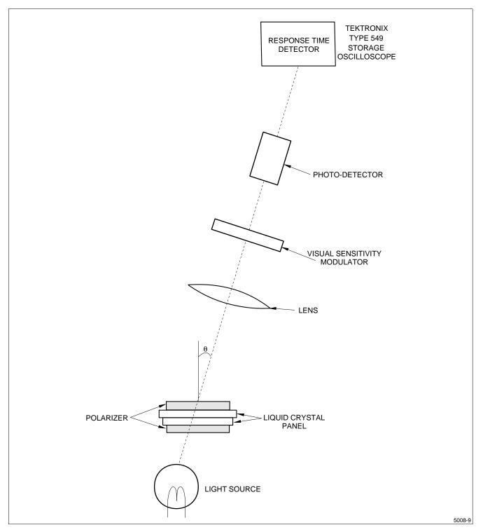
Figure 9. Optical Characteristics Test Method II
