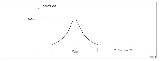
Figure 8. Definition of  $V_{MAX}$
